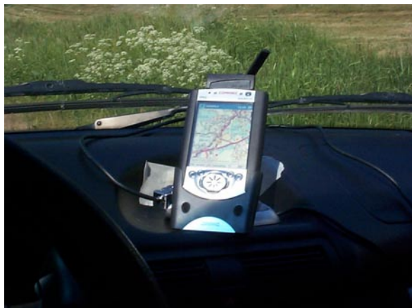
Figure 8 –SISNeT handheld receiver installed inside a car during preliminary tests
