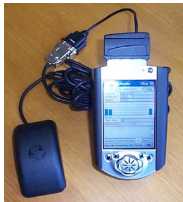
Figure 6 – SISNeT handheld receiver based on an iPAQ PDA: Hardware configuration during development
