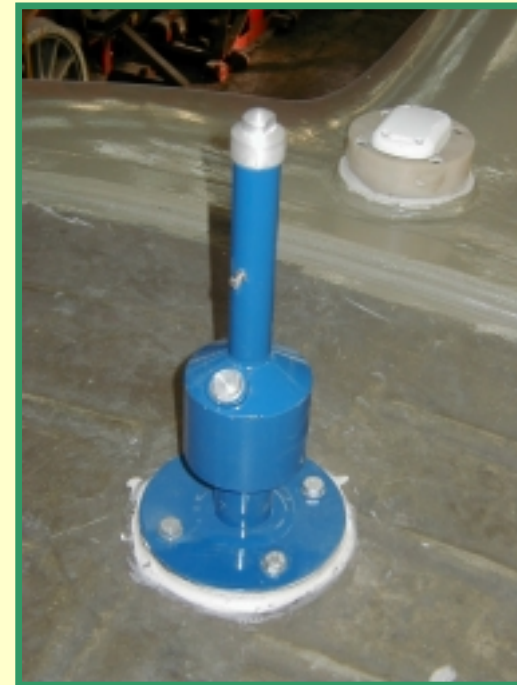
The radio modem and GPS/GLONASS antennas on the roof of the 130 023-5 locomotive.
