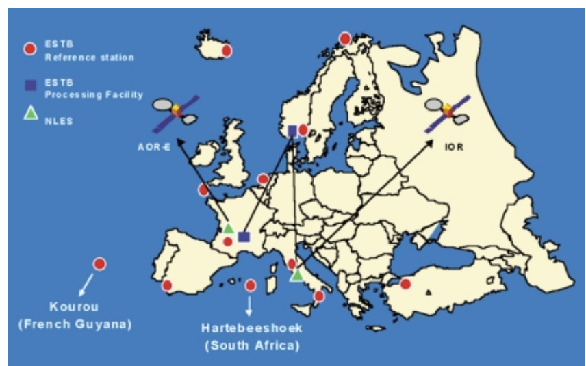
Figure 6. The EGNOS System Test Bed (ESTB) architecture
