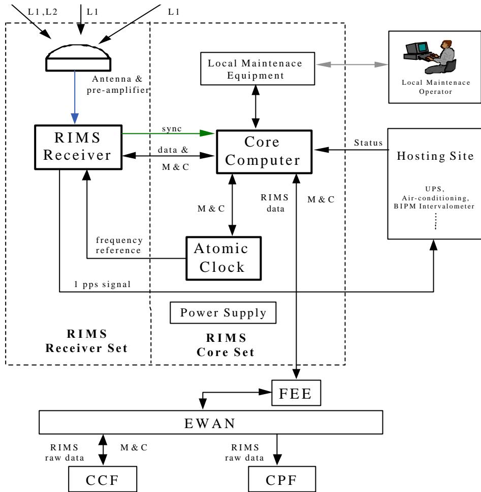
**Fig 2 Example of a RIMS channel architecture**
