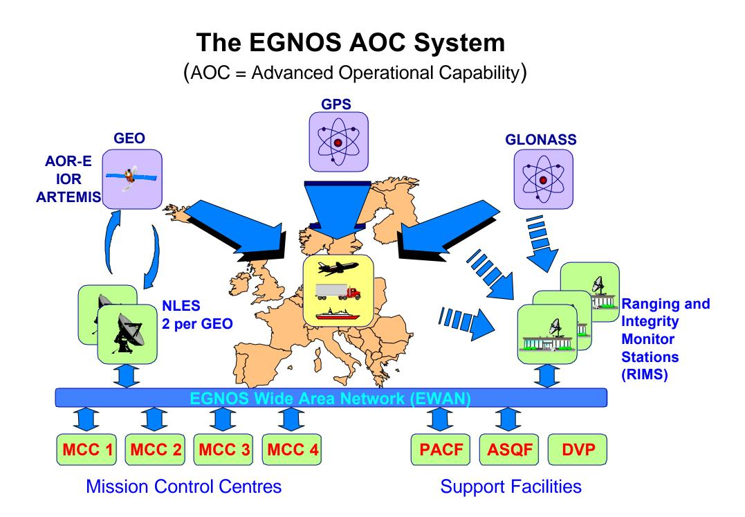
EGNOS Augments GPS and GLONASS Performance for multi-modal Users For Civil Aviation Users it will support operations in all phases of flight down to CAT-1 Precision Approach
