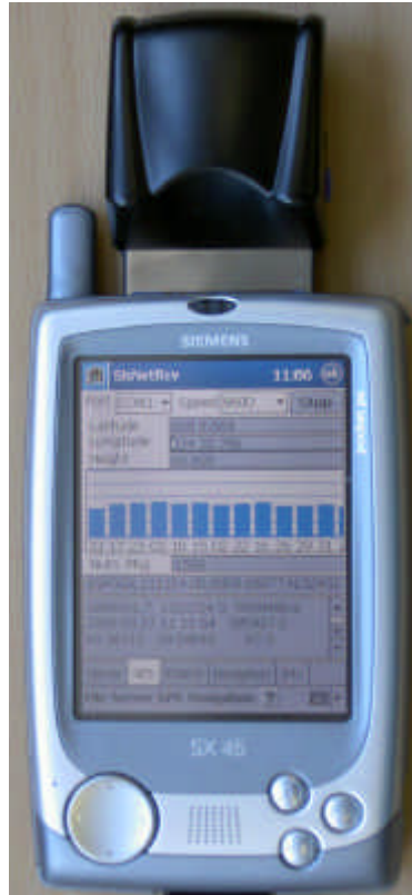
Figure 8 - SISNeT handheld receiver embedded into a mobile phone
