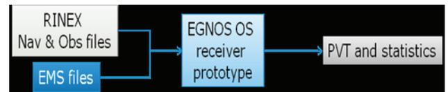
Figure 2 EGNOS OS receiver prototype interfaces overview.
