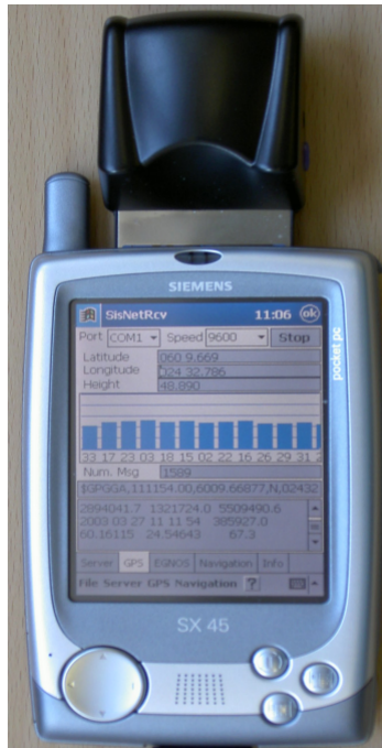
Figure 1 - SISNeT handheld receiver embedded into a mobile phone
