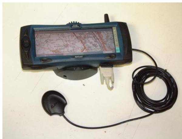
Figure 2 – SISNeT handheld receiver based on a NetPad device, for experimentation in urban buses in Toulouse (France).
