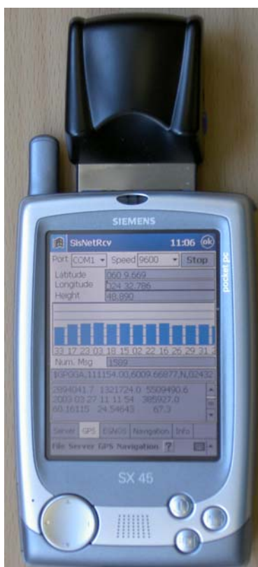
Figure 8 - SISNeT handheld receiver embedded into a mobile phone
