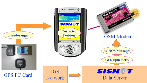
Figure 2. SISNeT handheld receiver (based on an iPAQ PDA)
