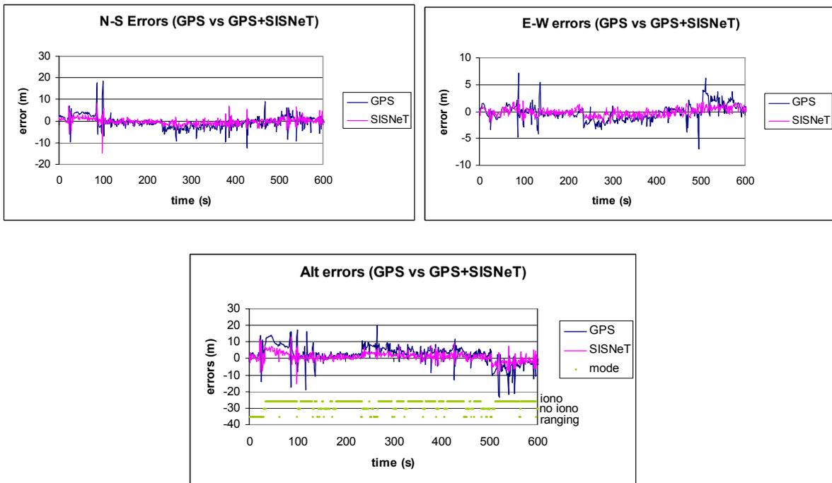
Figure 7: Dynamic test with ShPIDER. North, East and Up errors comparing GPS and GPS+SISNeT.
