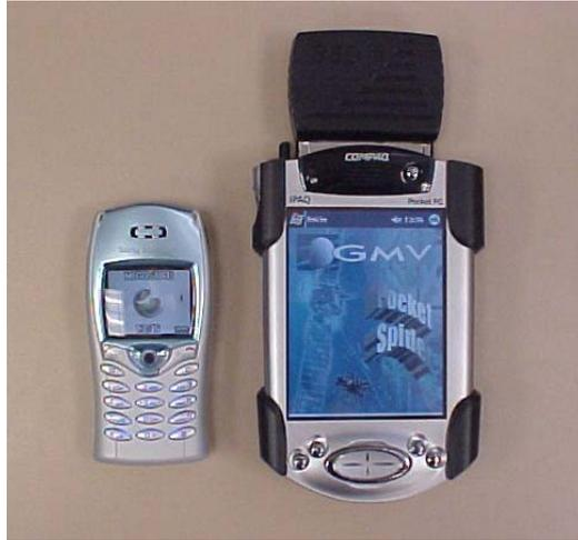
Figure 12: Complete System: Ericsson T68i, iPAQ H3970 with Pocket-ShPIDER application and EMTAC PCMCIA GPS receiver.
