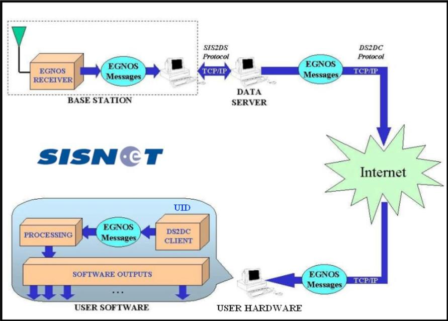
Figure 1: Overall architecture of the SISNeT system.
