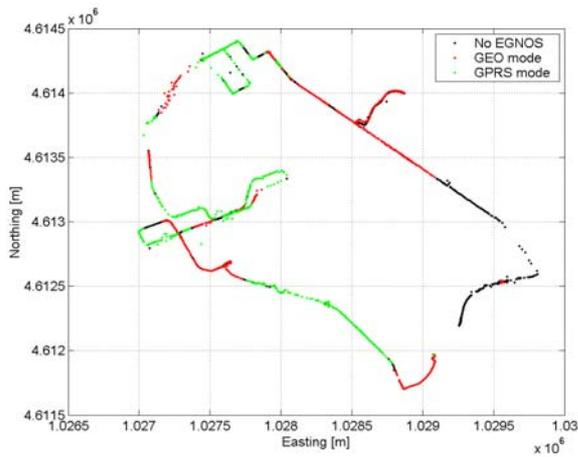
Figure 10: EGNOS TRAN trajectory (red and green lines indicating the availability of SBAS corrections)
