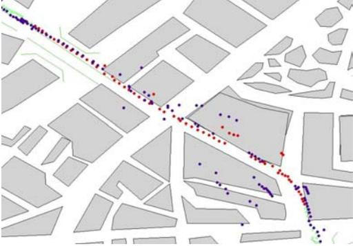
Figure 9: SISNeT (red) vs. GPS (blue) tracks in an urban environment. Results from urban bus tests in Valladolid.
