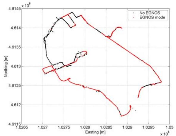
Figure 11: ShPIDER trajectory (red line indicating the availability of SBAS corrections)
