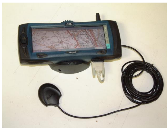
Figure 3 –SISNeT handheld receiver based on a NetPad device, for experimentation in urban buses in Toulouse (France).
