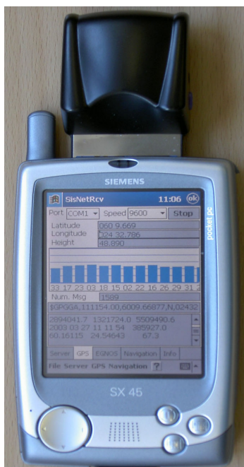
Figure 2 - SISNeT handheld receiver embedded into a mobile phone
