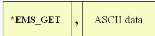
Figure 3. Format of the *EMS_GET message. For each EMS_GET command sent to the Data Server, the user receives a set of *EMS_GET answers, containing the requested information. 4
