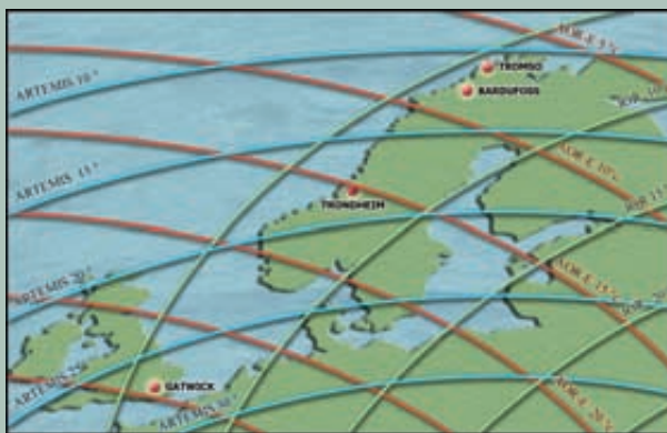
High latitude flight trial locations showing geostationary satellite elevation angles.
